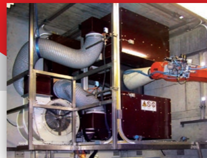
Removing magnetism from parts for electron beam welding application. Compensation for the earth's field is done by using 3D-Helmholtz coils.
