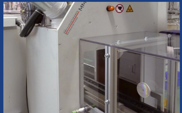
An MM VE with an integrated light barrier for pulse activation, allowing the machine to operate completely automatically.
